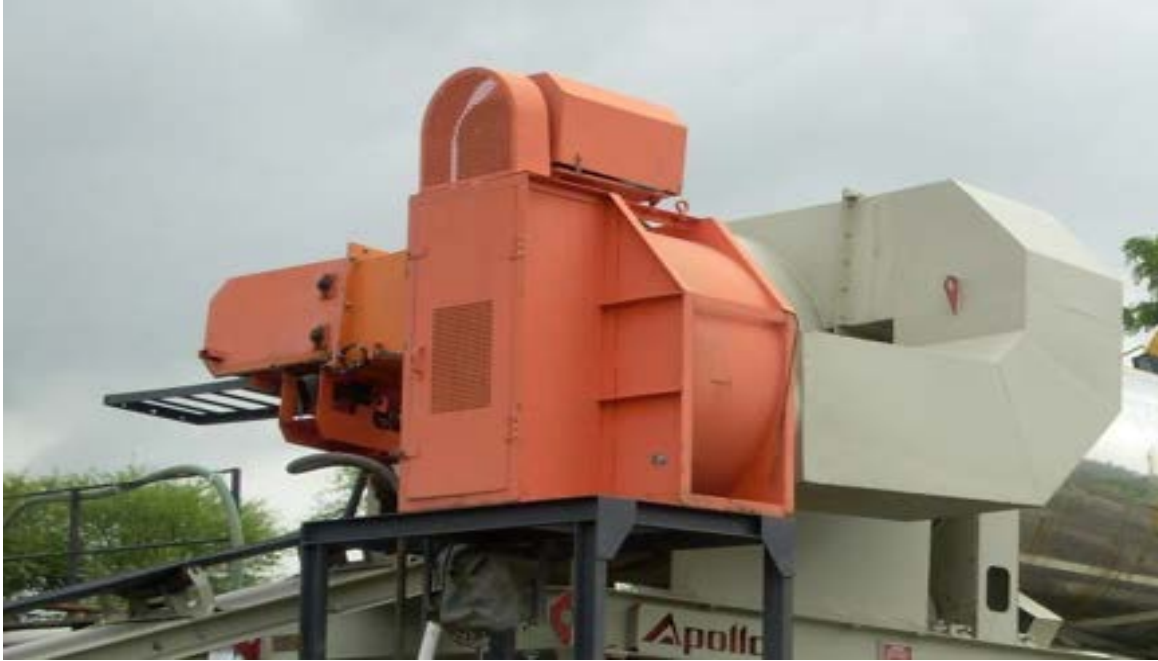
Fig. Aggregate Dryer
