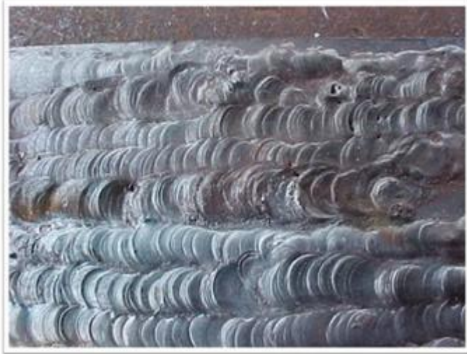
Figure 7.23 unacceptable weld profiles
