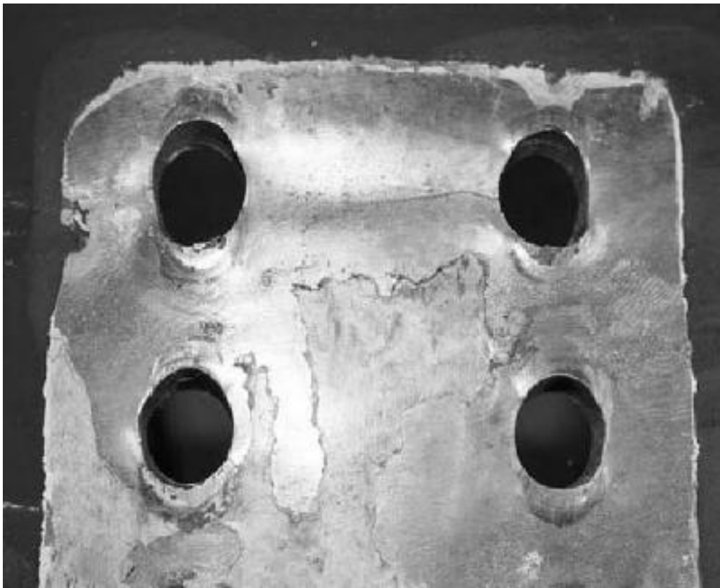
Figure 10.16 Bearing failure of plates
